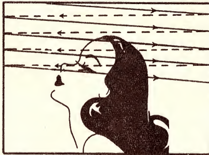
Figure 1. An elementary scanning pattern. The solid lines represent the scanning movement, the dotted lines the retrace action. The distance between the lines is exaggerated to simplify the drawing.
